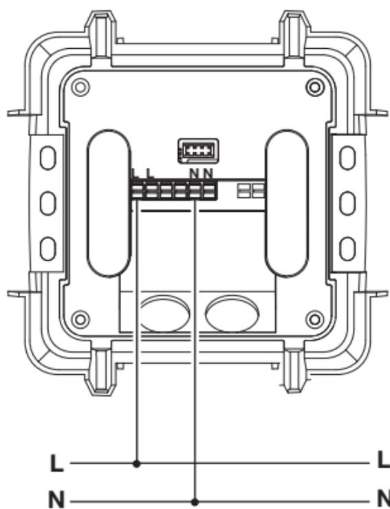
The power supply line consists of a 2- or 3-core cable:
